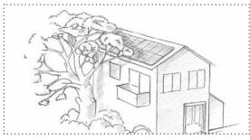
Partial shading is no longer an issue. With conventional string inverters, partial shading usually affects the entire system and so adversely impacts yield. But with a micro inverter system, modules that are not affected continue to operate at top performance.
