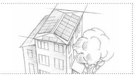
Does your roof face in different directions? Here too, a feed-in system comprising individual inverters is the solution: Uneven irradiation conditions may even be of advantage because energy can be consumed more efficiently and throughout the day.
