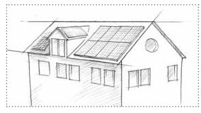
The independently operating modules enable optimum usage of all roof surfaces – whether dormers, eaves or a surplus module with an odd number. Even string-based systems can be easily expanded.
